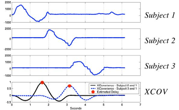
**Figure 2. Raw data for hands raised and lowered in sequence (only the pitch gyro is shown) and resulting average cross-covariance.**
