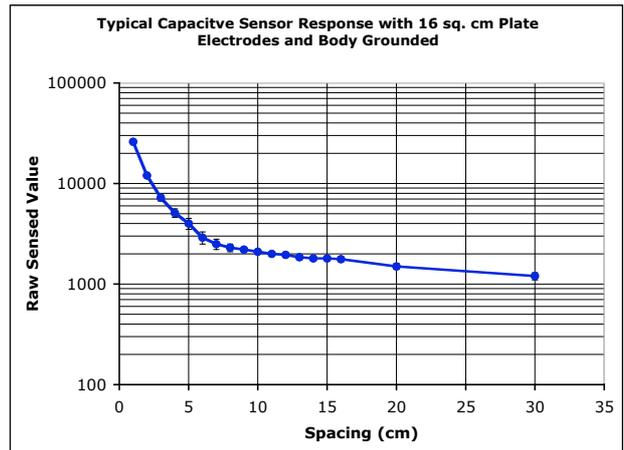
**Figure 8. Typical response of the capacitive sensing system.**
