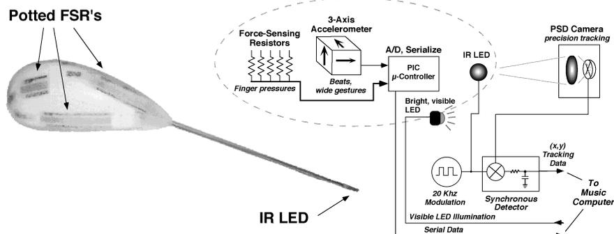
Figure 1: The Digital Baton; Photograph (left) and Schematic (right)
