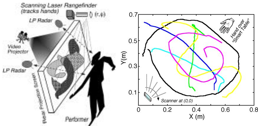
Figure 3: “Smart Wall” and hand trajectory measured by triangulation rangefinder
