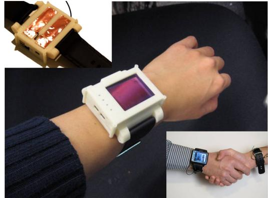
Figure 8: The Wrist Sensor Unit
