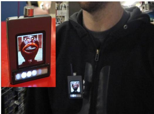
Figure 7:  $\mu$ Badge Wearable Device Pinned to a User
