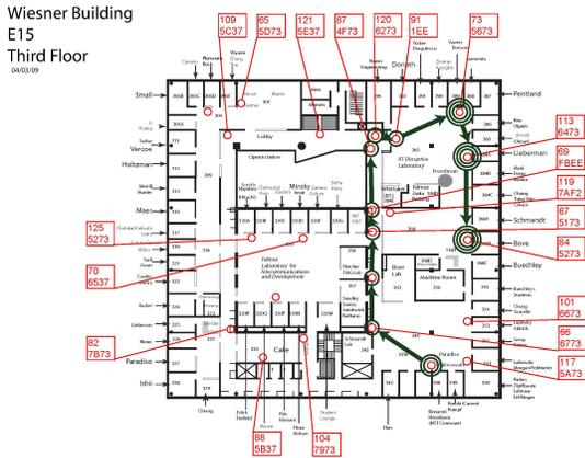
Figure 9: Trajectory of Participant relative to cameras during 1-hour test run
