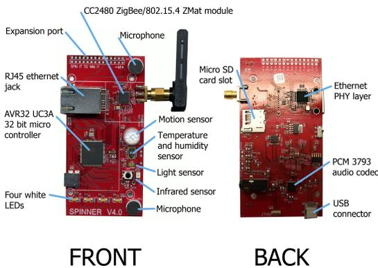
Figure 3: Sensor Node from Distributed Sensor Network, "The Red Board"
