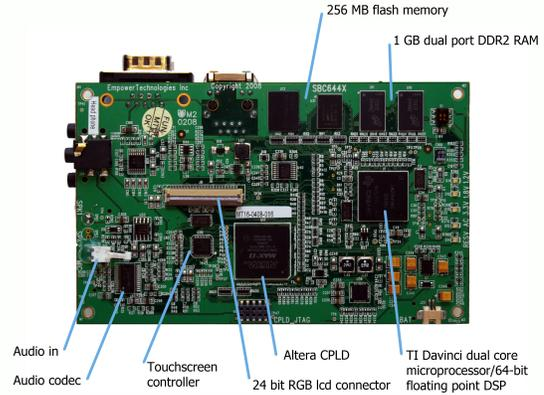
Figure 4: Embedded Audio Video Capture and Processing Device, "The Green Board" (front)
