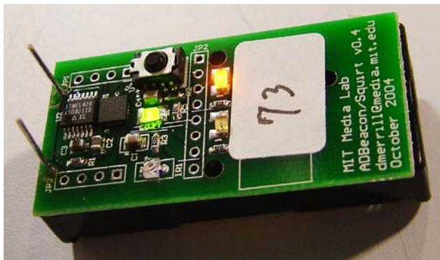
Figure 4. The "Squirt" - a compact IR tagging beacon
