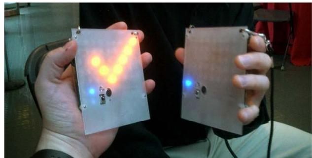
**Figure 6. The badge at right has bookmarked the badge at left - blue LEDs signify an encounter in progress and the checkmark verifies the bookmark. Note that this early version of the badge lacked the easier-to-use front-mounted buttons and only used the side-mounted switch.**
