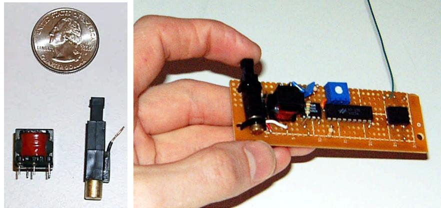
**Fig. 2.** Critical components (left – not including US quarter) and operational prototype board (right) for self-powered wireless ID pushbutton transmitter of Fig. 1
