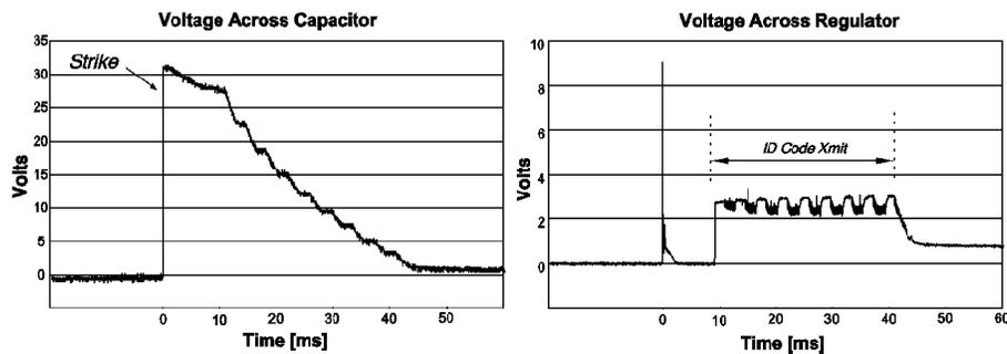
**Fig. 3:** Voltage across tank capacitor and regulator output voltage vs. time for a single press
