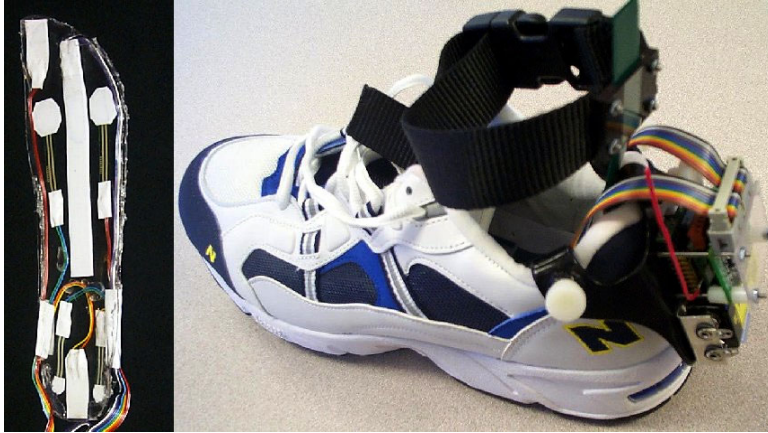
Figure 2: Photos of the first prototype of the SIGSS – insole (left) and shoe with electronics (right)
