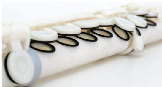
Fig. 7. A picture of the Objet flute's printed pads (soft material in black), printed simultaneously with the flute body and key mechanisms (rigid material in white).
