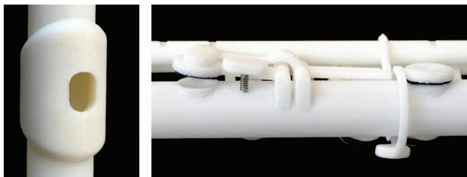
Fig. 5. A picture of the FDM flute's mouthpiece (left) and a key's mechanism, using metal spring (right).
