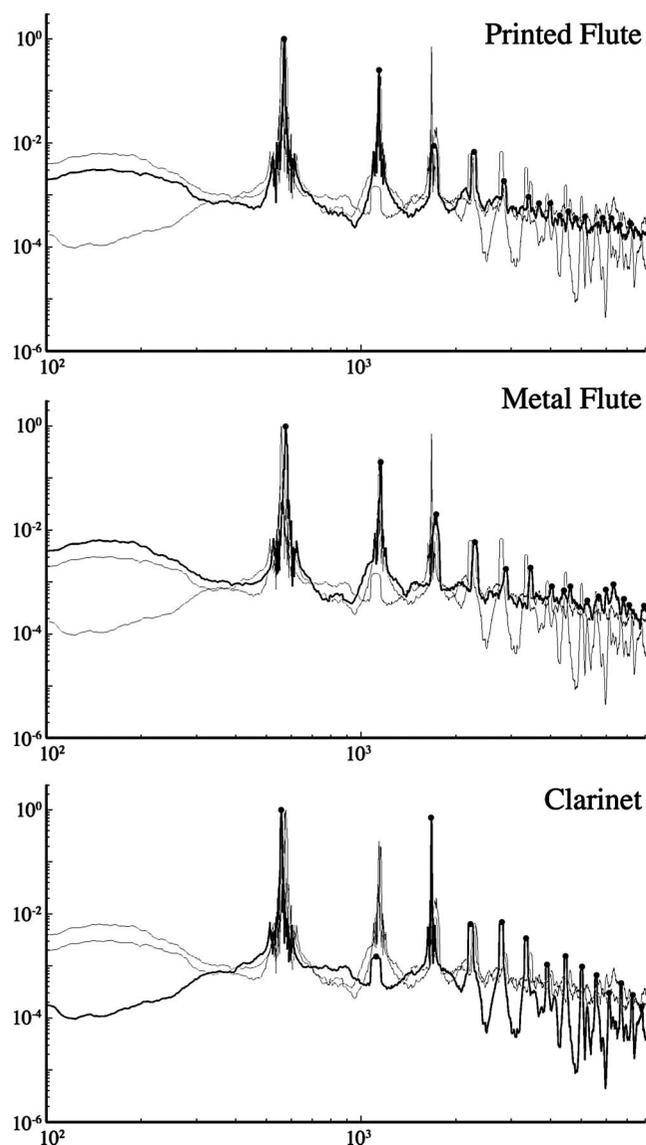
Fig. 8. Logarithmic spectrum comparison of the B1 note, based on recordings of a length of 0.3 s which do not include the transient, of a printed Objet's flute (top), a regular metal flute (middle), and a clarinet (bottom). In each plot the grey graphs are the two other recordings, for reference. The clarinet sound sample was taken from [www.compositiontoday.com](http://www.compositiontoday.com), and was not recorded under the exact same conditions.
