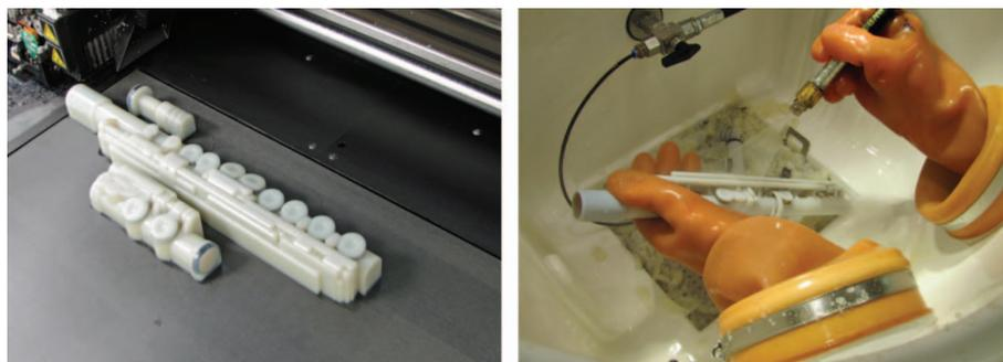
Fig. 2. Printed flute parts by Objet Connex500, covered with support material (left), and the cleaning process (right).
