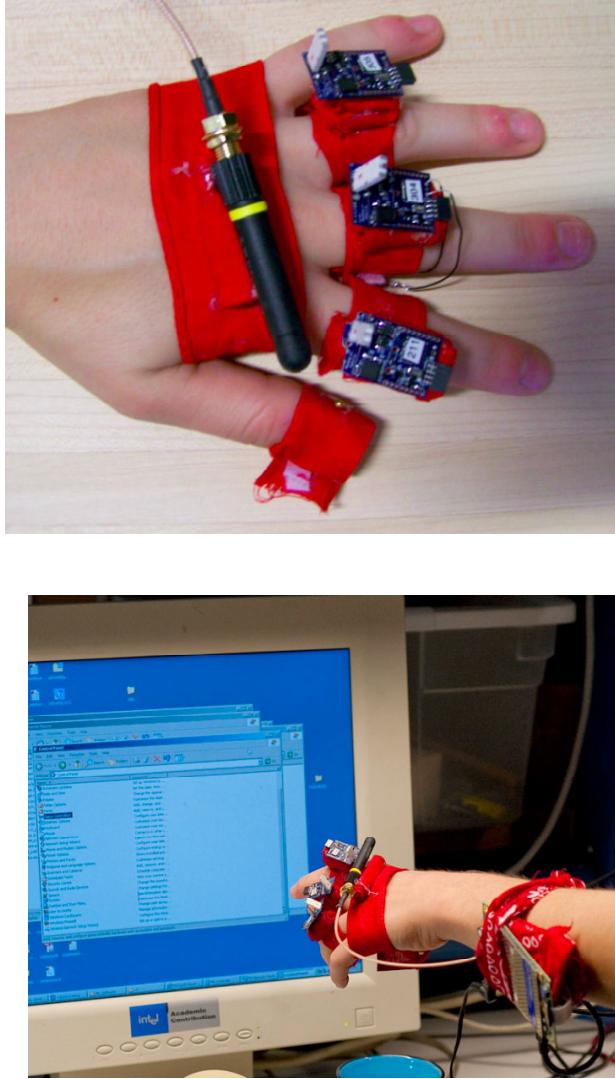
Figure 2. Our prototype system on a user's hand (top) during tests (bottom).
