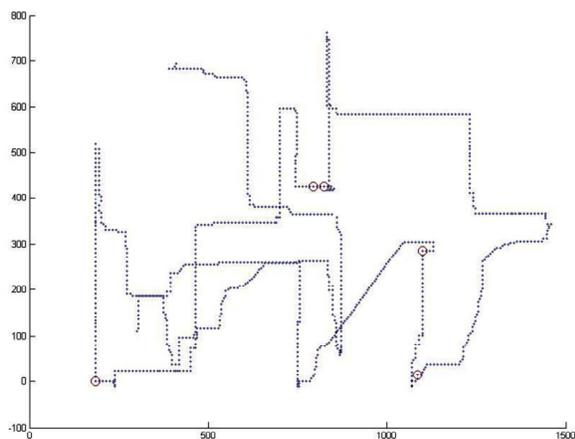
Figure 4. Actual mouse trace (plotted in pixels) for a user manipulating their index finger to scroll around the GUI screen. Clicks are denoted by circles. This is an XY plot of the data shown in Figure 3.
