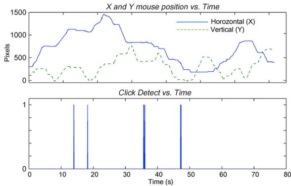
Figure 3. Processed mouse tracking coordinates (top) and click data (bottom) vs. time for a user interacting with the GUI application.
