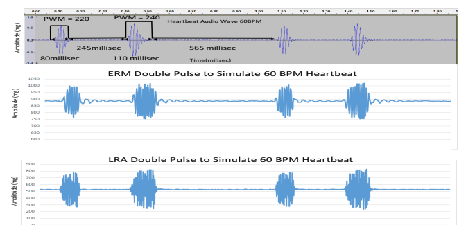
Figure 4. Heartbeat audio (top) and acceleration of a reference mass produced along x axis by an ERM (middle) and long z axis by an LRA (bottom)
