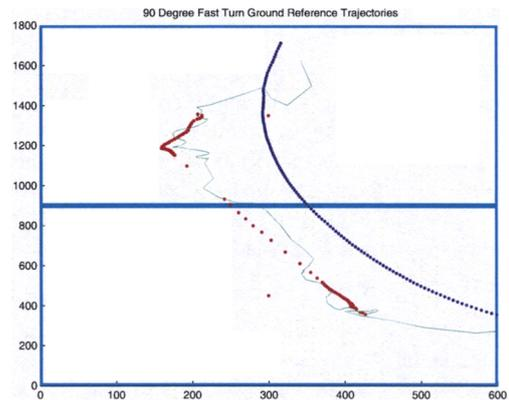
Fig. 5: Depicted above are the two force-plates with the ground reference trajectories, CM (blue), CMP(green), COP(red). The walking direction is from the top of the picture down.
