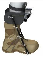
**Fig. 1** Active autonomous ankle exoskeleton. The active autonomous ankle exoskeleton used a winch actuator on the shin to actuate the proximal ends of fiberglass struts attached to the boot. The winch actuator implemented a brushless DC motor and pulley transmission to wind a high strength cord. The motor controllers and batteries were worn around the chest and waist. Reflective markers on the strut were used to measure the deflection of the struts and the applied exoskeletal torque
