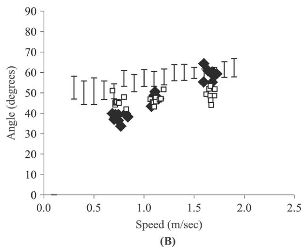
**Note:** Using the non-adaptive, mechanical knee (plot A, filled diamonds) and the adaptive knee (plot B, filled diamonds). As in Figures 6 and 7, the subject's sound side leg is shown (open squares), along with reference data from unimpaired walkers (standard error bars). In both (A) and (B), maximum flexion angle is low compared to the biological data except at the fastest walking speed
