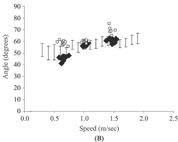
**Note:** Using the non-adaptive, mechanical knee (plot A, filled diamonds) and the adaptive knee (plot B, filled diamonds). In (A) and (B), the subject's sound side leg is shown (open squares), along with reference data from unimpaired walkers (standard error bars). In (A), the peak angle increases with increasing speed, exceeding seventy degrees, but in (B) the maximum flexion angle is less than seventy degrees and is in reasonable agreement with biological data
