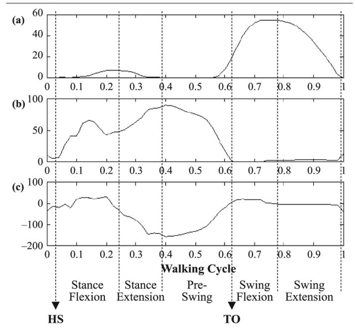
**Figure 5** Adaptation of swing-flexion damping at a constant forward walking speed
