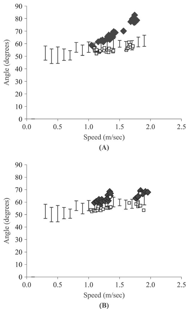
**Note:** Using the non-adaptive, mechanical knee (plot A, filled diamonds) and the adaptive knee (plot B, filled diamonds). In (A) and (B), the subject's sound side leg is shown (open squares), along with reference data from unimpaired walkers (standard error bars). In (A), the peak angle increases with increasing speed, far exceeding seventy degrees, but in (B) the maximum flexion angle is less than seventy degrees and agrees well with biological data
