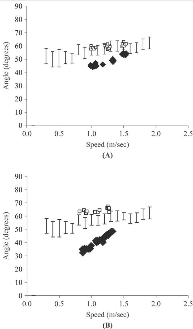
**Note:** Using the non-adaptive, mechanical knee (plot A, filled diamonds) and the adaptive knee (plot B, filled diamonds). Here again, the subject's sound side leg is shown (open squares), along with reference data from unimpaired walkers (standard error bars). In both (A) and (B), maximum flexion angle is low compared to the biological data even at the fastest walking speed
