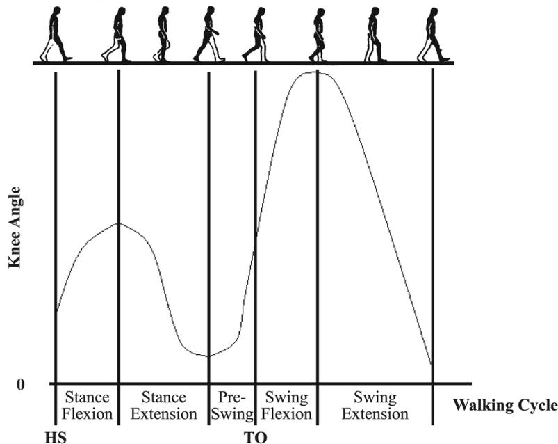
**Note:** State 1 and State 2 represent early stance flexion and extension just after heel strike (HS), respectively. State 3, or pre-swing, typically occurs at the end of stance, beginning just after the knee has fully extended and terminating when the foot has left the ground at toe-off (TO). State 4 and State 5 represent periods of knee flexion and extension during the swing phase of walking, respectively
