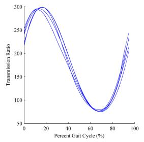
Fig. 2. The convergence of the MCMM on the optimal transmission ratio profile is depicted above. The five transmission profiles that resulted in the lowest energy consumption are shown. The subject was waking at 1.5 m/s and 0% gait cycle corresponds with heal strike.
