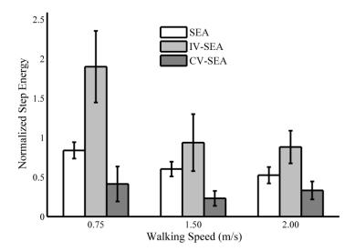
Fig. 3. The step energy of each transmission actuating a knee prosthesis was estimated for three different subjects walking at three different speeds. The step energy was normalized by the step energy required by a direct drive actuator.
