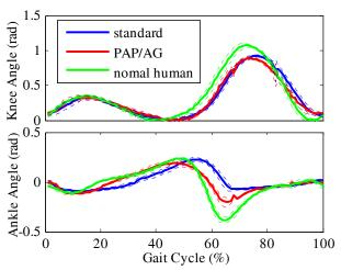
Fig. 9 Knee and ankle angle of trials with standard prosthesis, PAP with AG, and normal human walking.
