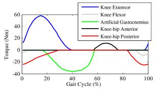
Fig. 3 Contribution from each spring. The Artificial Gastrocnemius (AG) works from the mid stance phase until toe off, similar to the biological gastrocnemius.
